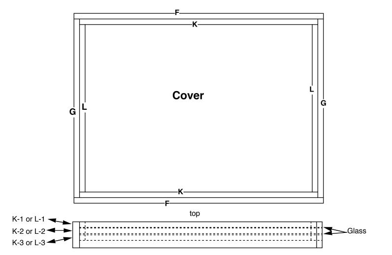
To Assemble fasten Gs & Fs as shown. Put on 2 Ks & 2 Ls flush with the top. Working from the bottom. Insert glass to rest on K & L then put another set of 2 Ks & 2 Ls then another glass & another set of Ks & Ls.
